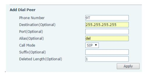
Figure 56 - Deletion Configuration
