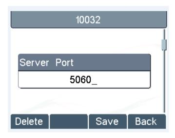
Figure 20 - Configure SIP Proxy Server Port
