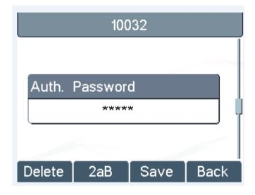
Figure 5 - Configure SIP Authentication Password
