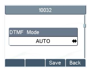
Figure 12 - Configure DTMF Mode
