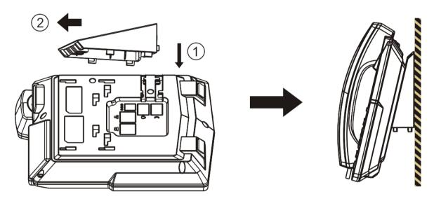
Figure 2 - Wall-mount Installation
