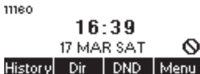
Figure 56 - DND Enabled on All Lines
