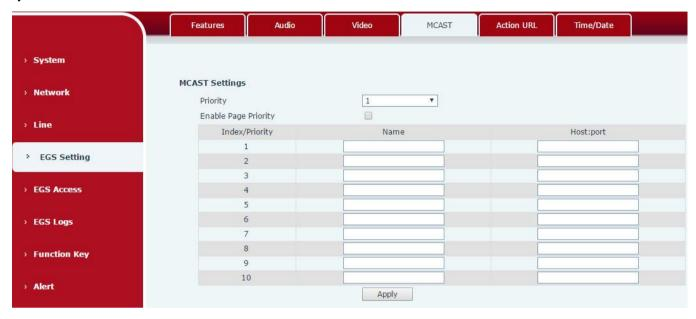
It is easy and convenient to use multicast function to send notice to each member of the multicast via setting the multicast key on the device and sending multicast RTP stream to pre-configured multicast address. By configuring monitoring multicast address on the device, monitor and play the RTP stream which sent by the multicast address.
