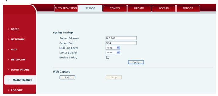
Syslog is a protocol used to record log messages using a client/server mechanism. The Syslog server receives the messages from clients, and classifies them based on priority and type. Then these messages will be written into a log by rules which the administrator has configured.
