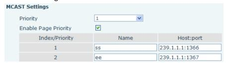
The multicast SS priority is higher than that of EE, which is the highest priority.
