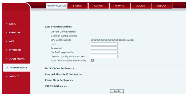
The equipment supports PnP, DHCP, and Phone Flash to obtain configuration parameters. They will be queried in the following order when the equipment boots.
