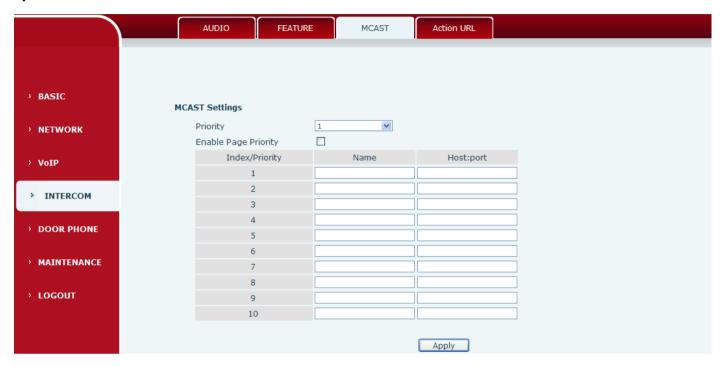
It is easy and convenient to use multicast function to send notice to each member of the multicast via setting the multicast key on the device and sending multicast RTP stream to pre-configured multicast address. By configuring monitoring multicast address on the device, monitor and play the RTP stream which sent by the multicast address.
