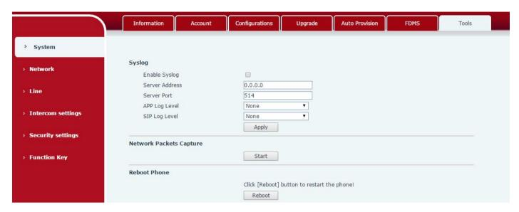
Syslog is a protocol used to record log messages using a client/server mechanism. The Syslog server receives the messages from clients, and classifies them based on priority and type. Then these messages would be written into a log by rules which the administrator has configured.
