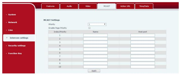
It is easy and convenient to use multicast function to send notice to each member of the multicast via setting the multicast key on the device and sending multicast RTP stream to pre-configured multicast address. By configuring monitoring multicast address on the device, the device monitors and plays the RTP stream which sent by the multicast address.
