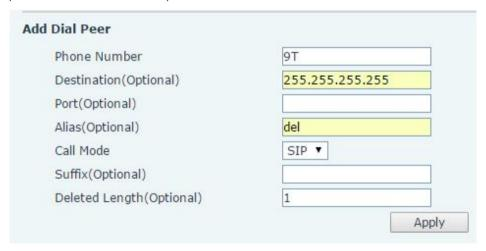
Figure 17 - Deletion Configuration
