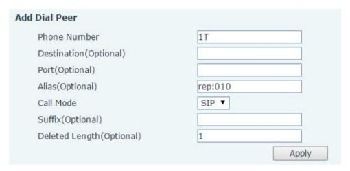
Figure 14 - Local Substitution Configuration
