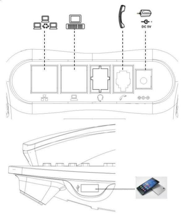
Figure 1 - Device to Connection
