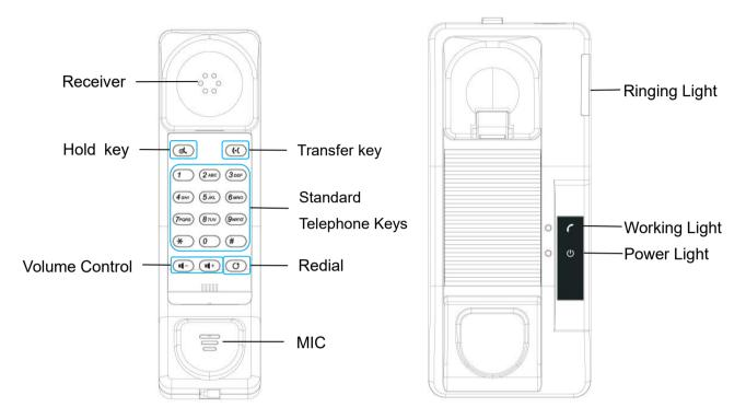
The above picture shows the keypad layout of the device. Each key provides its own specific function. User should refer to the illustration in this section about the usage of each key and the description in this document about each function.
