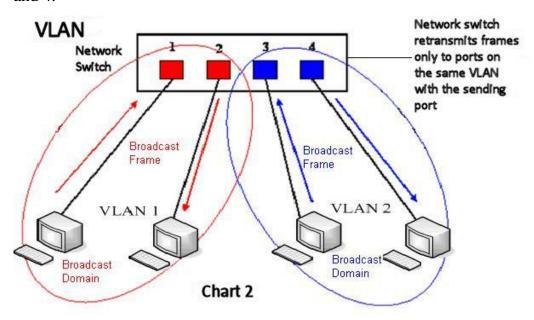
Chart 2 shows an example with two VLANs indicated by red and blue. In this example, frames broadcast from Port 1 will only go to Port 2 since Ports 3 and 4 are in a different VLAN. VLANs can be used to divide a network by restricting the transmission of broadcast frames.
